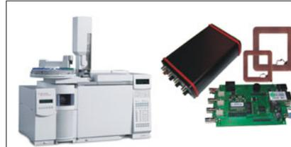
Sample is automatically analysed with the method info from the TAG. No user interaction or sequence setup required. Report and results stored in LIMS system.
