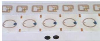
The integration of small RFID tags (such as our 20mm square 13.57 MHz inlays) onto drug boxes, cases and pallets together with the use of our special bulk-tag RFID terminals allow operators to detect and locate multiple boxes at a time. Through these tagging and serialization a complete solution could manage all of the manufacturer, wholesaler and pharmacy's processes.
